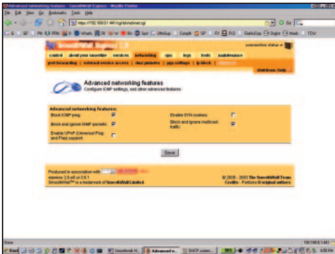
■ HERE YOU CAN CHECK TO BLOCK ICMP PINGS, IGMP PACKETS AND MULTICAST, IF YOU SO DESIRE.
