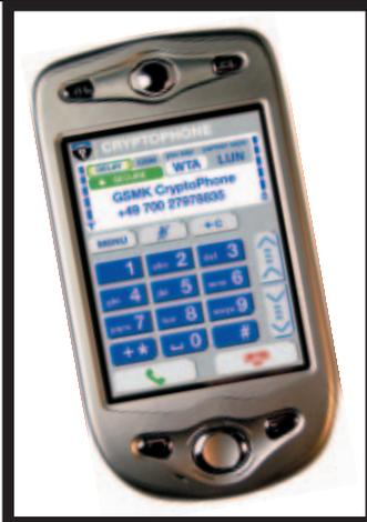
LEFT: The GSMK CryptoPhone 200, the world's first secure PDA-based cellular phone.
